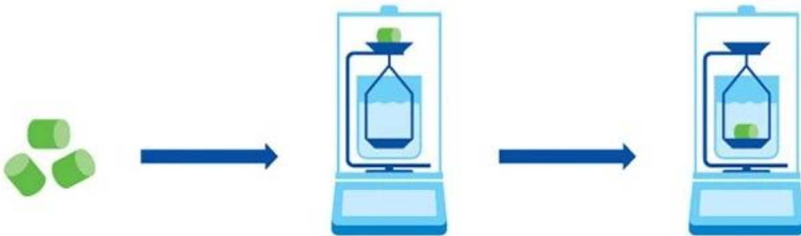
Figure 1. Density measurement of a test specimen according to BS EN ISO 1183-1
